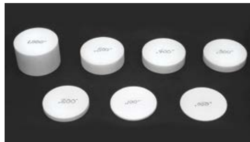
Calibration spacer set 26U-51U (0.050, 0.100, 0.200, 0.300, 0.400, 0.500, 1.000) 850859-001
